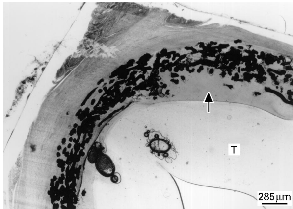
Figure 6 Histological section showing part of the fibre mesh porosity filled with the silicone glue (arrow) used to attach the fibre mesh cuff to the silicone tube (T).
